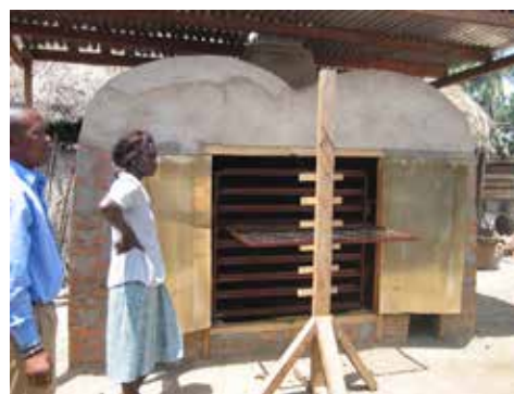
FIGURE 17 AFSMO-150 improved fish smoking kiln in a fishing village near Accra, Ghana
