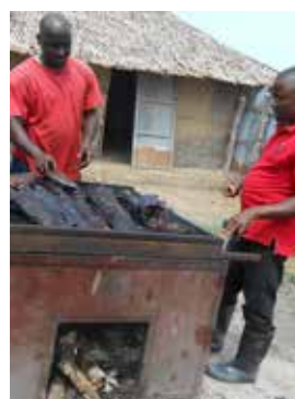
FIGURE 16 Detachable and portable single compartment Banda for flood-prone areas in the Congo
